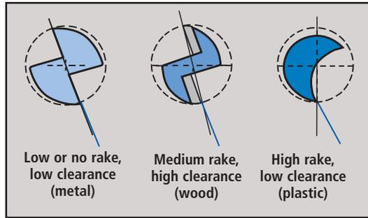
Figure 1: Tool geometries for metal, wood and plastic.
